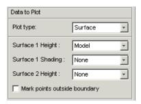
You can view any of these options alone as a primary surface (by leaving the last two options set to None). You can add a second option to shade the primary surface, for example to color your model surface with the error between the model and the strategy, to highlight problem areas.
