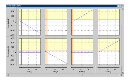
The Left Value is compared with a plot of the Right Value output on the same axes. This comparison is illustrated for the table gradient example problem. Consider the top-left graph in the figure shown. Constraint4(1) is the first Left Value  $(rg_1^{inc})$  of the table gradient constraint in the example problem. Recall that this can be written as
