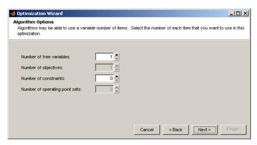
The foptcon algorithm can only have a single objective, so this control is not enabled. Choose the number of free variables and constraints you require. You can also add constraints later.
