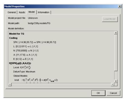
Here you can view the model definition, the project file, and the model path. Function model definitions are shown here. For MBC models the model definition (showing the parameters and coefficients of the model formula) is the same information you would see in the Model Browser part of the toolbox when selecting **View > Model Definition**.
