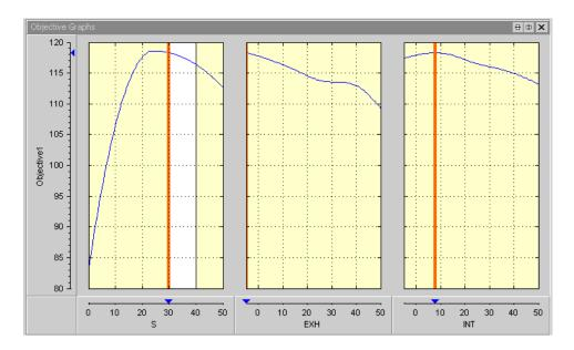
The Objective Graphs show cross-section plots of the objective function against each free variable in the problem. The left plot is a plot of the objective function against S, with EXH and INT at their optimal values, for the second run. The range constraint for the second operating point (30  $\leq$  S  $\leq$  40) can be seen; within the constraint region is white, and all other regions outside the constraint are yellow.
