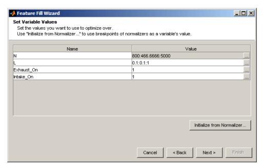
• You can edit normalizers manually, or you can click the **Initialize From Normalizer** button to reach a dialog box where you can select normalizers and interleave values between breakpoints. Interleaving values can minimize interpolation error by adding values between each normalizer value. In this way you can create a grid of more points than table cells to optimize over. Select normalizers in the dialog box to use those breakpoints as a variable's value.
