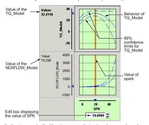
Performing a tradeoff calibration necessarily involves the comparison of two or more models. For example, in this case, the tradeoff allows a calibrator to check that a value of spark that gives peak torque also gives an acceptable value for the NOX flow model.
