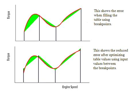
To see the difference between optimizing table values and optimizing the positions of breakpoints, compare with the illustration in "Optimizing Breakpoints" on page 4-22.
