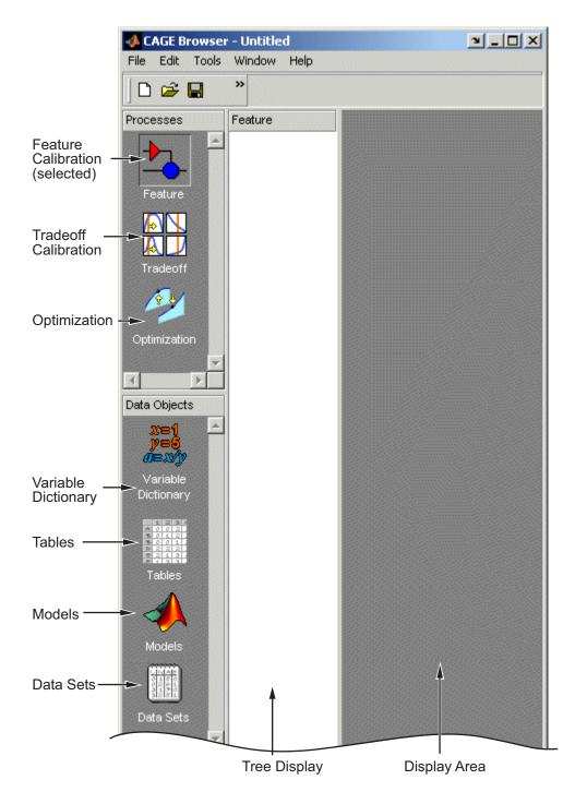
CAGE includes a **Processes** pane and a **Data Objects** pane to help you identify the type of calibration you want to do and the data objects that you intend to use. Use the buttons in these panes to navigate between the different sections of functionality in CAGE.
