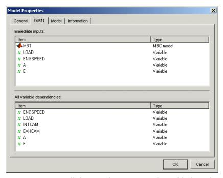
Here you can view all the immediate inputs and variable dependencies of your model. For some models the two lists will be the same; in the example shown one of the inputs is another model (MBT) so the variable dependencies list also shows the variable inputs for that model. This information is shown graphically in the **Connections** pane.
