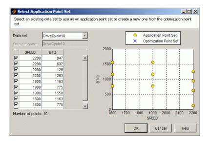
**4** View the plot displaying the application points and optimization points. CAGE extrapolates the optimization results to evaluate the objective or constraint at the application points.
