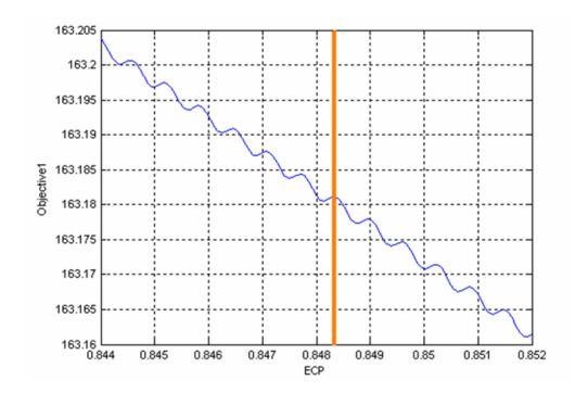
You can see that the model is noisy and the optimizer has (correctly) returned a local maximum of the model. However, this result is a maximum of the noise component in the model and not the physical component. If the noise is not behavior of the physical system, then you should remodel the noisy models in the Model Browser. The CAGE Import tool can be used to replace the noisy models with the results of the remodeling and the optimization can be rerun.
