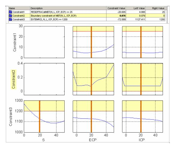
These constraint views confirm that Constraint2 is violated for this run. Therefore, this solution is probably best left as unacceptable. In cases like this, if it is not already marked as unacceptable, clear the **Accept** box in the Optimization Results table for this run.
