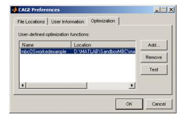
The example shows the worked example function, which is already registered with CAGE for use in the optimization tutorial.
