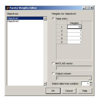
In this dialog box, you can select objectives to sum, and select weights for any run by clicking and editing, as shown in the previous example. The same weights are applied to each solution to calculate the weighted sums. Click **OK** to apply new weights, and the weighted sums are recalculated.
