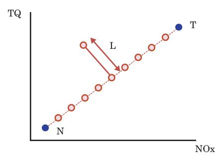
The figure above shows spacing of the points between the along the (n-1) surface. The algorithm tries to maximize the distance L along the normal away from the surface. The following figure shows the final solution found by the NBI algorithm.
