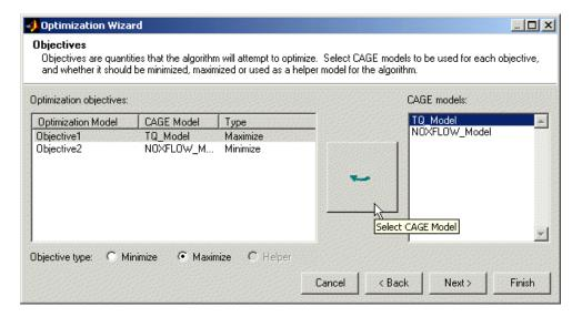
Here you can select which models from your session you want to use for the optimization, and whether you want to maximize or minimize the model output. The foptcon algorithm is for single objectives, so you can only maximize or minimize one model. The NBI algorithm can evaluate multiple objectives. For example, you might want to maximize torque while minimizing NOX emissions. Remember you can also define constraints later, for example, using emissions requirements.
