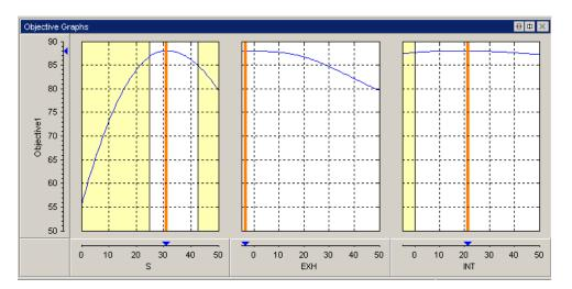
The objective slice graphs show the objective functions at the point selected in the table, with the solution value in orange. Whether the table is displaying a solution slice or pareto slice, the cell you select in the table is always displayed in the graphs. The objective graphs show cross section plots of the objective function against each free variable in the problem.
