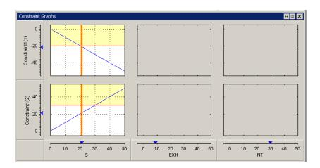
The constraint graphs for a range constraint shows how the Left Value of each output of a range constraint depends on the free variables in the optimization. The Left Value is compared with a plot of the Right Value output on the same axes. This comparison is illustrated for the example problem at the second run, as shown in the top left graph.
