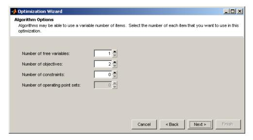
NBI must have a minimum of two objectives, and you can choose as many free variables and constraints as you like. You can add constraints later if required.
