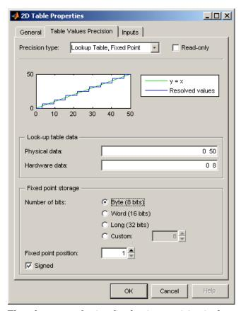
The advantage of using fixed-point precision is the reduction in computation needed for such numbers. However, it restricts the numbers available to the user.
