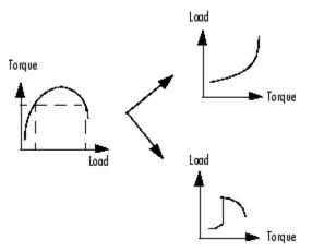
The process of inverting a one-dimensional table is different from the process of inverting a two-dimensional table.
