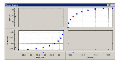
You can use the Pareto Front graphs, shown in the preceding figure, in combination with the table views (Solution Slice and Pareto Slice) and the other plots in the graphs (Objective Slice and Constraint Slice graphs) to help you select best solutions for each run. You can collect these solutions together in the "Selected Solution Slice" on page 7-35.
