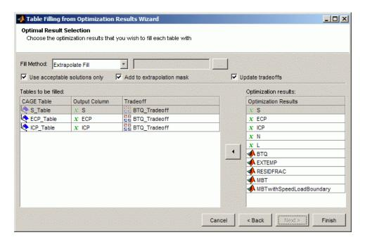
In a single objective optimization there is only one solution for each operating point. In a multiobjective optimization there is more than one solution per point, so you must first select the preferred solutions before you can use the Table Filling wizard. To collect your preferred solutions you must use the "Selected Solution Slice" on page 7-35, then you can use this wizard to fill tables with the selected solutions.
