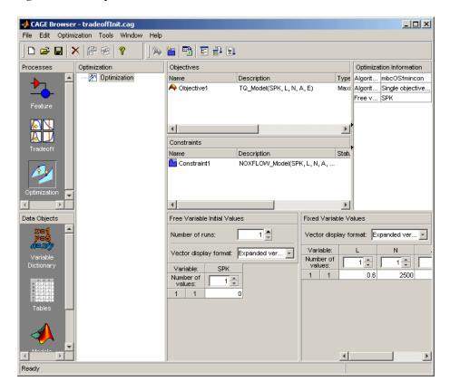
If your optimization is ready to run you can click **Run Optimization** in the toolbar to proceed. You may want to edit variable values, constraints or objectives before running the optimization. If you need to set up any objectives or constraints **Run** will not be enabled. If your optimization is ready to run you can also click **Set Up and Run Optimization** if you want to change algorithm-specific settings such as number of required solutions and tolerances for termination.
